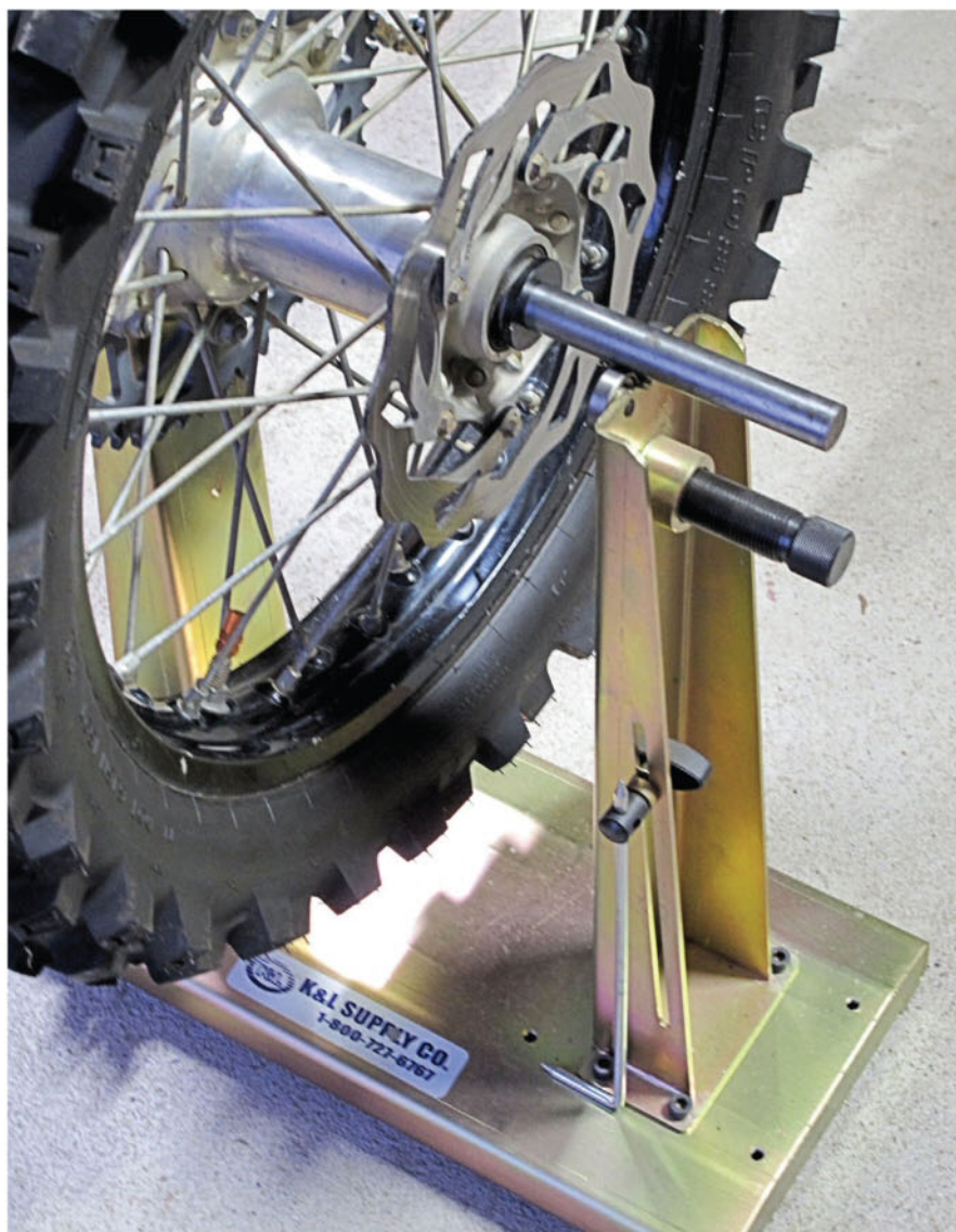
This balancing stand has a movable arm (lower right) for truing wheels. When in use, it swings up with its tip near the rim, making lateral and radial runout easily visible when the wheel is held between the threaded black posts (to prevent lateral movement of the hub). An out-of-round wheel will not balance properly.
